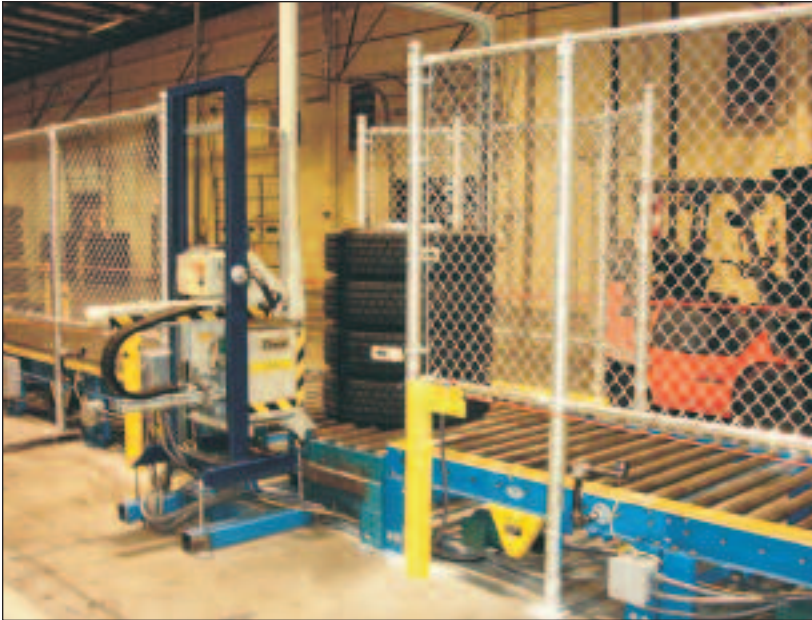
PAC installation of automatic conveying and strapping system for truck tires.
